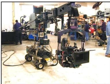
T-15 With Stab-C Mounted on Fisher 10
